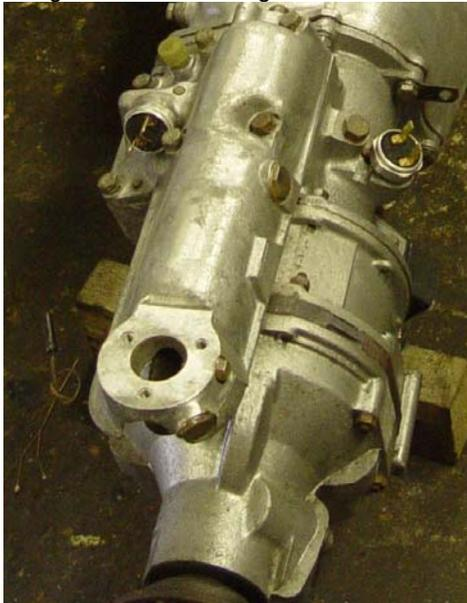
Circular opening at the back of the gearbox is for the gear lever which connects with the end of the remote control shaft that transmits the gear lever movements to the selector plate when you select gear. On either side of the gearbox are the twin terminals of two switches – on the offside the reverse light switch and on the other the overdrive isolation switch. (Photo: Gavin Bailey)
